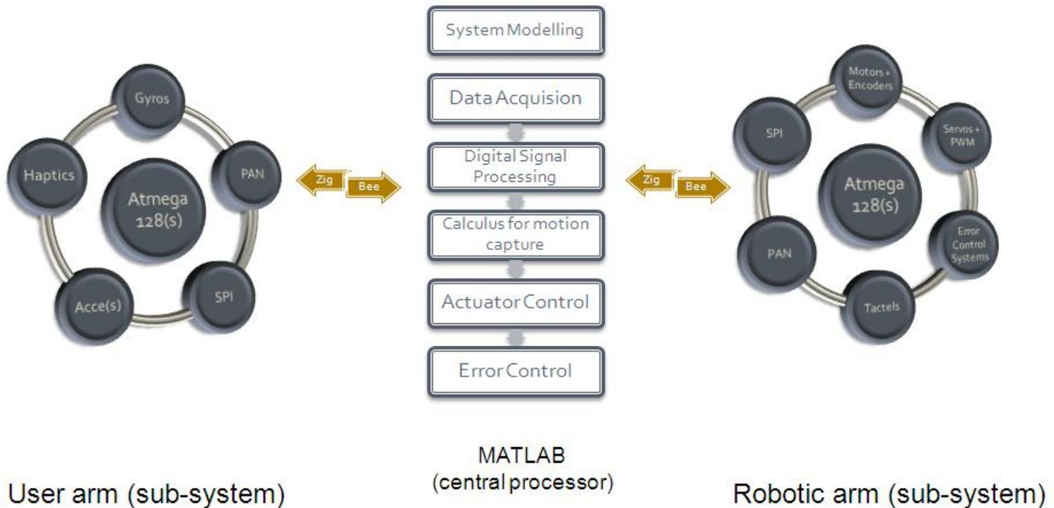
The physical system is divided into two broad halves – the user arm and the robotic arm. From the point of view of software, the system consists of a central processing station (MATLAB) and the two subsystems: user arm and robotic arm.
