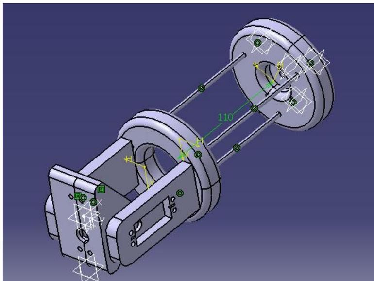
The elbow joint is replicated by a 2 axes design similarly powered by closed loop actuator systems:
